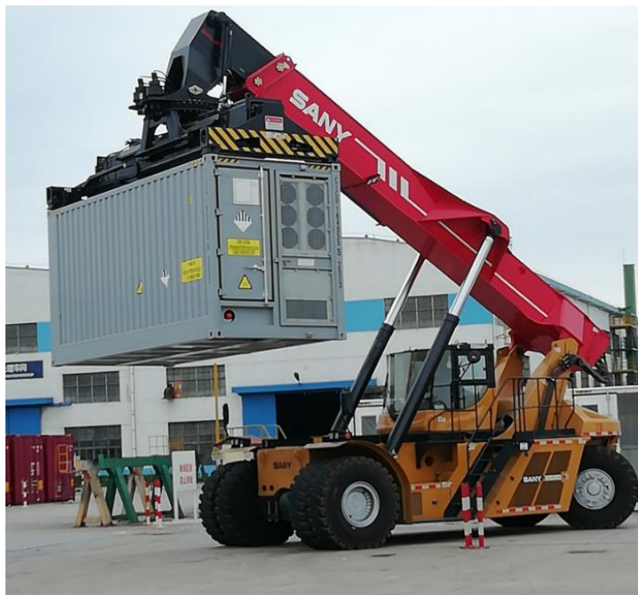
SDJ450: SANY classic spreader Rated capacity: 45t Application: ISO 20'/40'/45' Containers
